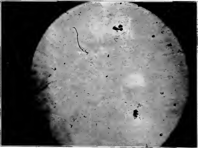
Photomicrograph of a .12% solution of Krabyn. The dark particles are often fragments of seed coats.
